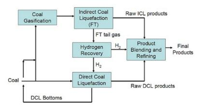
This hybrid liquifaction process map shows the significance of the gasifier (image courtesy DOE/NETL).
