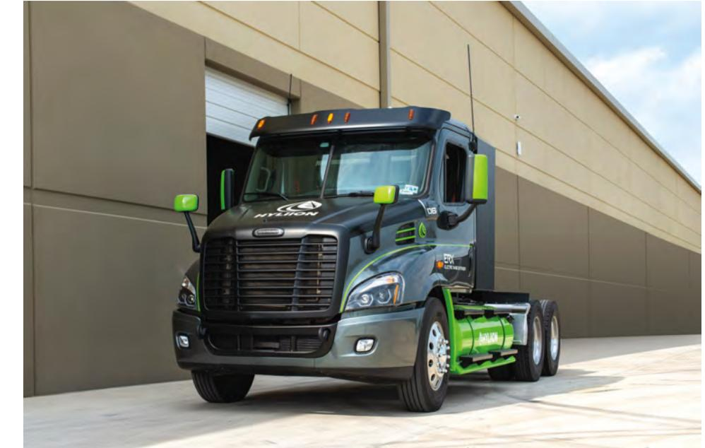
> **Hyllion** launched a fully electric, long-haul powertrain: the Hypertruck Electric Range Extender (ERX), which leverages an existing fueling infrastructure to offer fleets net-negative GHG emissions and low operating cost. With an electric drivetrain and a natural gas-powered onboard generator to recharge the battery, the Hypertruck ERX provides more than 1,000 miles of range.
