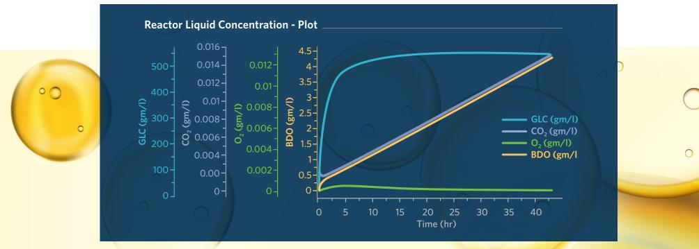
Figure 2. Aspen Plus generated composition plot shows the liquid phase concentration changes within the reactor through the reaction time. GLC here refers to the concentration of glucose as it builds up in the reactor.
