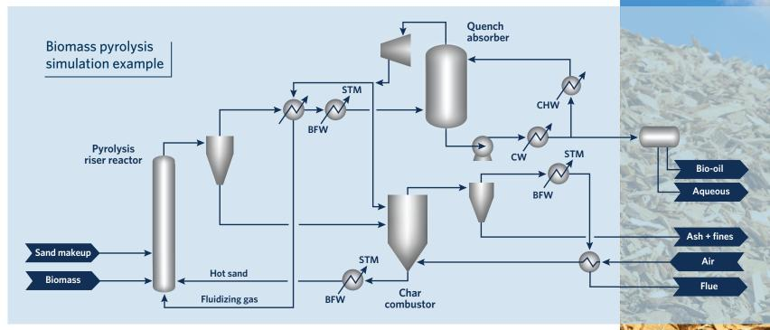
Figure 3. Biomass pyrolysis simulation example.
