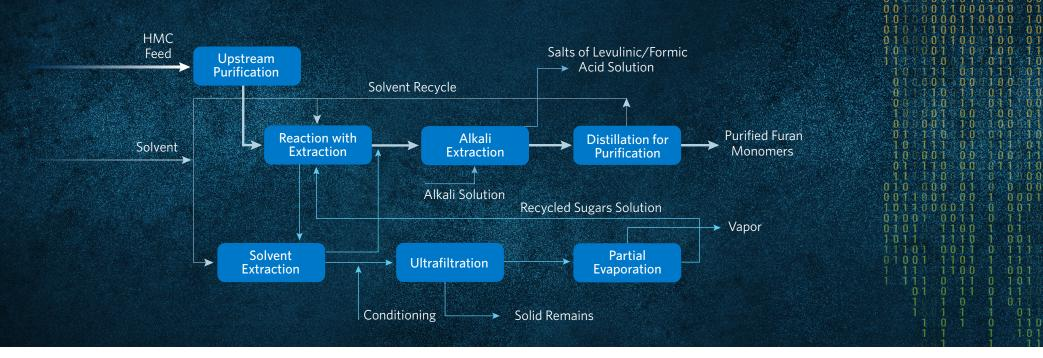
Figure 4. BioSprint process to convert hemicellulose to furan monomers.
