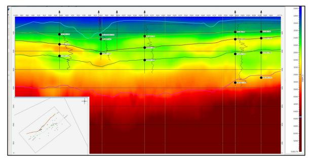
Fig.3c Final Interval velocity with sonic log
