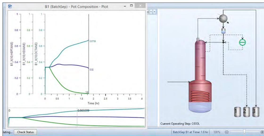
Figure 1: New dynamic plots capture time-lapse profiles or snapshots. Smart flowsheets animate during a run.
