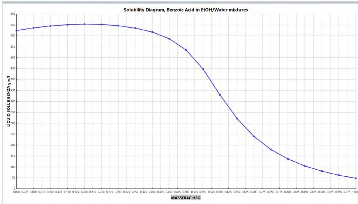
Figure 5: The new Solubility Analysis tool available starting in V10 of Aspen Plus
