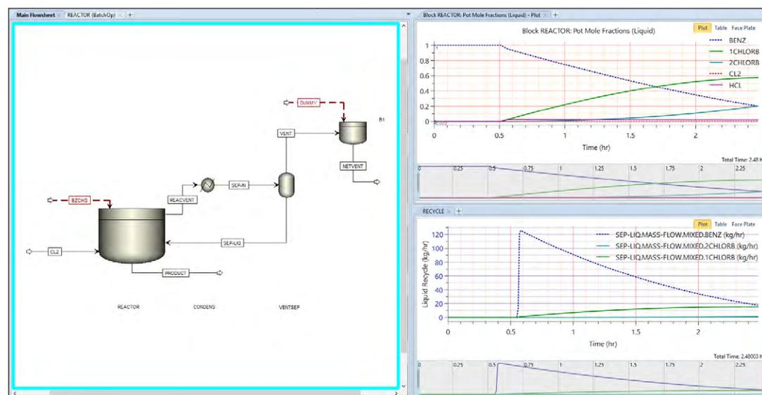
Figure 2: New plotting capabilities were added with the new BatchOp unit operations, including the ability to flip between plot and table views of results.
