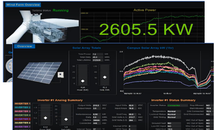
Figure 2. Detailed displays of renewable generation assets, including real-time values, trends integrated with historical data and alarm conditions.
