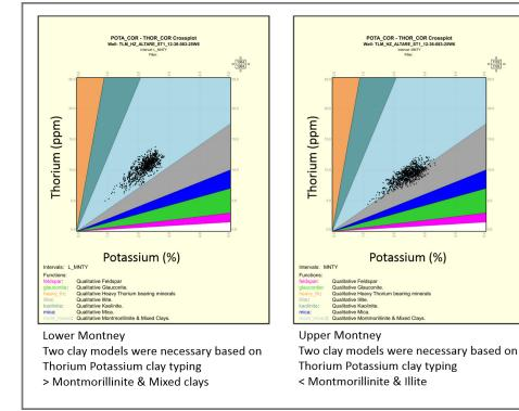
Figure 1. Montney Formation clay quantity and clay typing done in Geolog Facimage.
