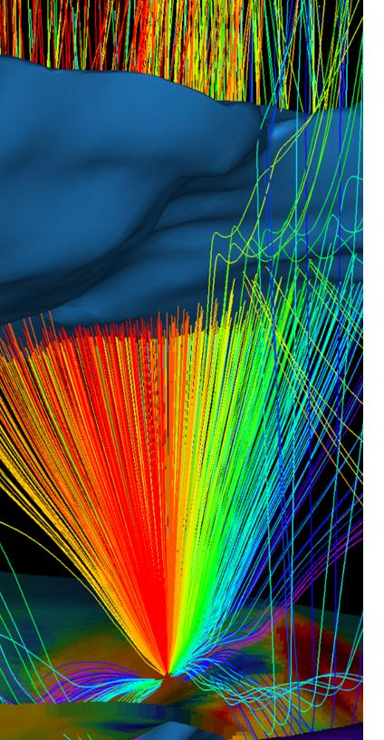
EarthStudy 360 reflection angle gathers provide "true amplitude" reflectivities that substantially increase the information needed to extract residual moveouts (RMO) and amplitude variations. The full-azimuth, angle domain RMO enables accurate velocity model determination (isotropy/anisotropy tomography). Full-azimuth, angle domain amplitude variations result in better reservoir characterization, with high-resolution elastic properties and high-resolution fracture determinations.
