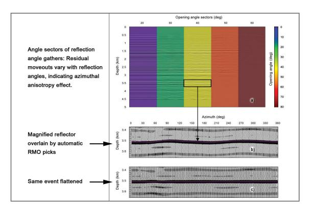
Angle sectors of reflection angle gathers: Residual moveouts vary with reflection angles, indicating azimuthal anisotropy effect.
