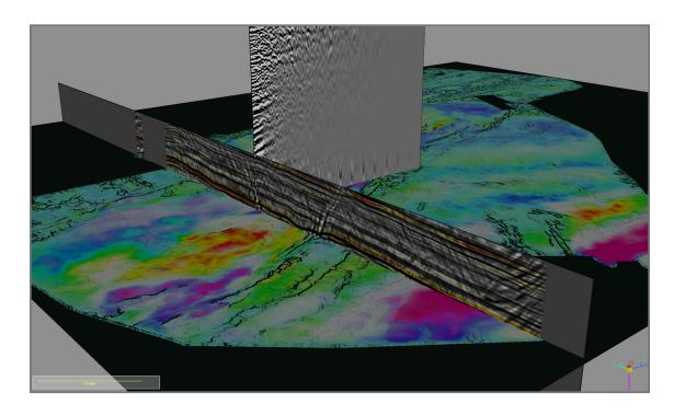
Highlight of fractures and faults using EarthStudy 360 diffraction imaging.
