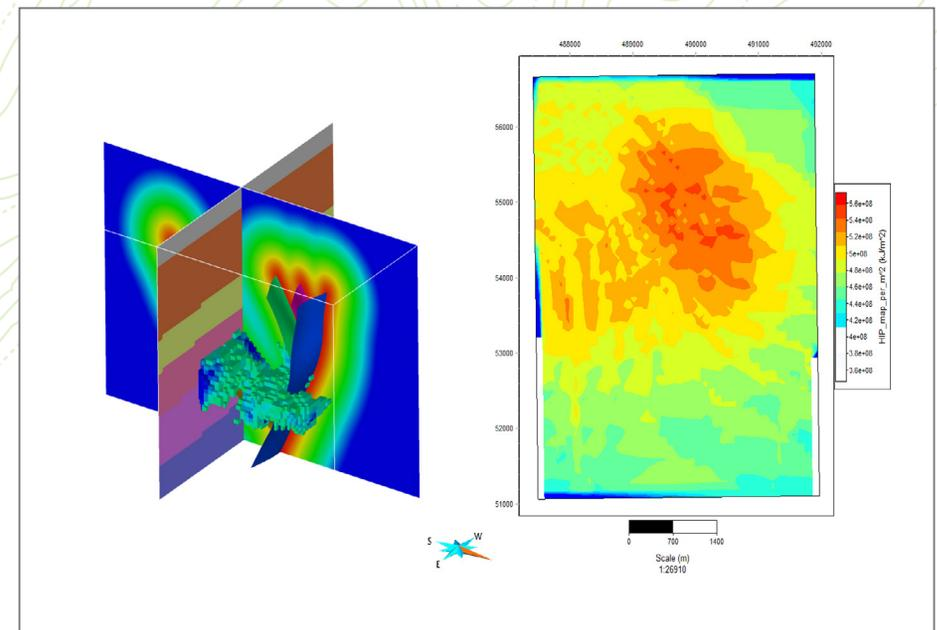
Figure 2. 3D play fairway analysis (left) and heat-in-place per m<sup>2</sup> map (right) of a geothermal field in SKUA-GOCAD.
